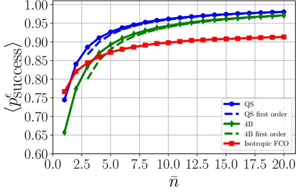
FIG. 3. Average success probabilities for our commuting-vs-anticommuting discrimination task of the QS, the 4B and the best isotropic FCO circuit, for  $1 \leq \bar{n} \leq 20$ . The connected points are obtained numerically for different values of  $\bar{n}$ , while the dashed lines (for the QS and 4B) are the analytical first-order expansions in  $1/\bar{n}$ , see Eqs. (28)–(29).
