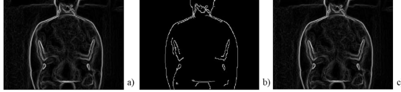
Fig.2. Example of gradient operators: a) Prewitt; b) Canny; c) Sobel
