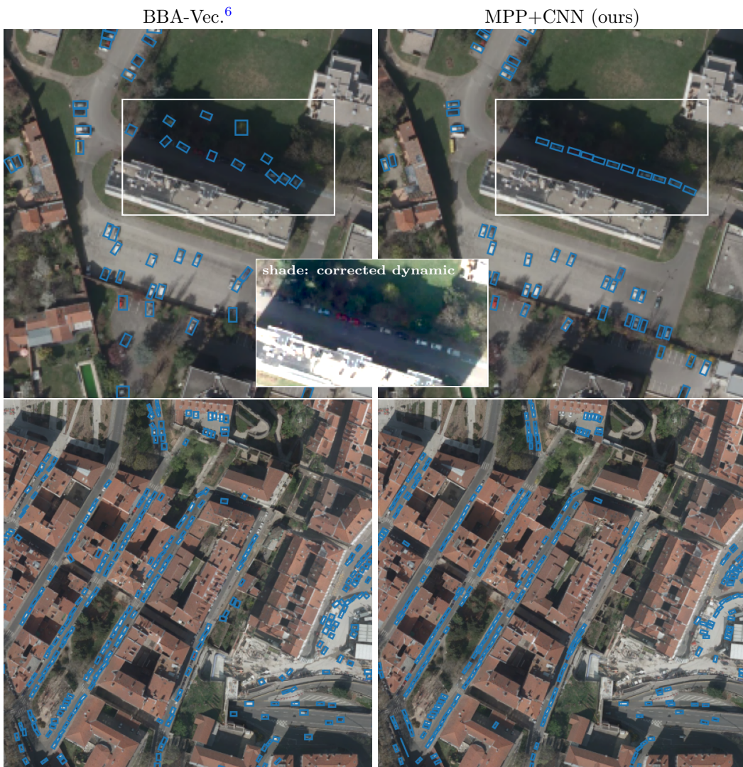
Figure 6. Detection results on samples of the data provided by Airbus, aerial photos subsampled to 50 cm/px, no ground truth available. [copyright Airbus Defense and Space]
