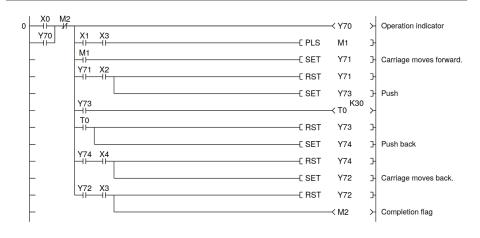
Fig. 2: Carriage line control: Ladder program.
