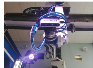
Fig. 5. The Intel D435 camera with a pan-tilt configuration.
