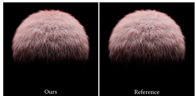
Figure 10: Hair rendering. We render the interreflection of light in this HAIRBALL asset containing 140k hair strands. The direct illumination is evaluated on the hull of the hair volume. We store the basis for the indirect lighting in textures using 10 texels per fiber (see Figure 11).
