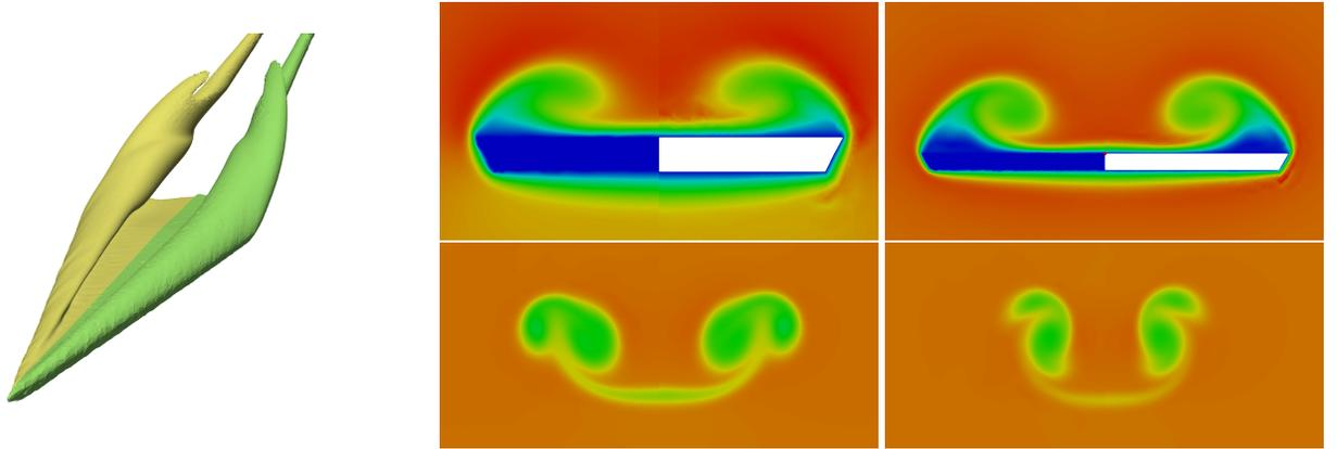
Figure 1: Laminar delta wing. **left** Roll-up of primary and secondary vortices. **right**  $\mathbb{P}^2$  Mach number distribution at  $x = 0.5C$ ,  $x = C$ ,  $x = 1.5C$  and  $x = 2C$ . In each picture on the left half the unfitted computation, on the right the body-fitted one.
