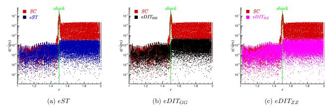
Figure 11: Transonic source flow: local discretization error analysis carried out on grid level 2 to compare the SC computations to the eDIT ones w.r.t.  $Z_4 = \sqrt{\rho}v$ .
