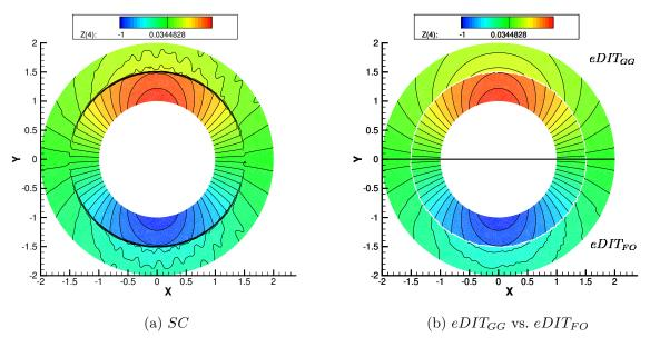
Figure 13: Transonic source flow: iso-contours comparison on grid level 2 w.r.t.  $Z_4 = \sqrt{\rho v}$ .
