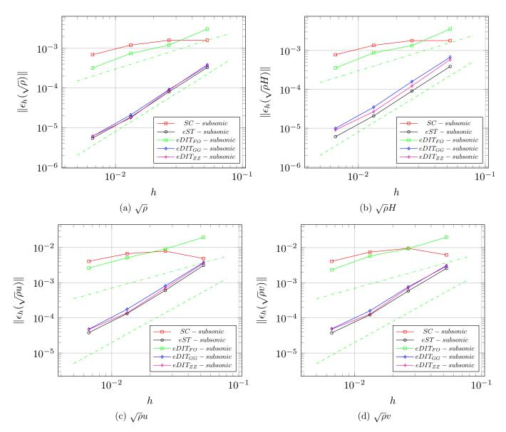
Figure 10: Transonic source flow: grid-convergence analysis within the shock-downstream (subsonic) region.
