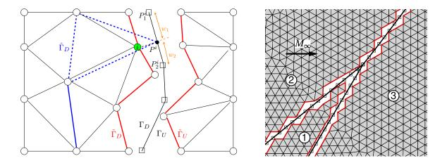
Figure 6: Left: auxiliary triangle defining the nodal gradient with corrected data on the front. Right: a problematic example of an interaction for which no auxiliary triangle can be built close to the interaction point in domain 1.
