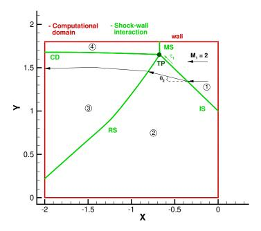
Figure 21: Mach reflection: sketch of the flow.
