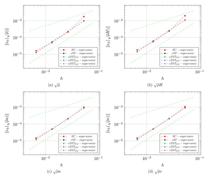
Figure 9: Transonic source flow: grid-convergence analysis within the shock-upstream (supersonic) region.
