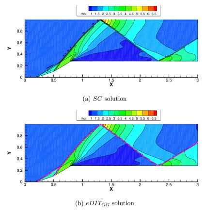
Figure 27: Supersonic channel flow: dimensionless density  $\rho/\rho_{\infty}$  iso-contours.
