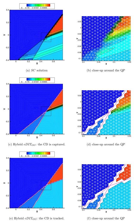
Figure 20: Interaction between two shocks of the same family: numerical solutions (comparisons in terms of  $S = p\rho^{-\gamma}$ ).
