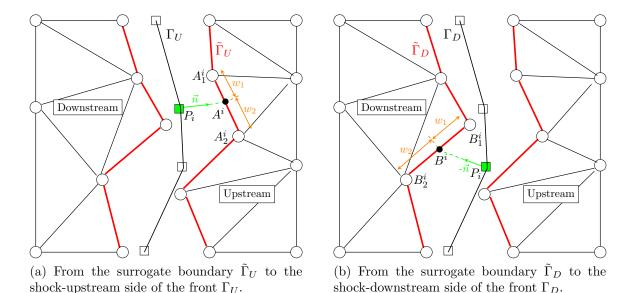
Figure 4: First transfer between the the surrogate boundaries and the front-mesh.
