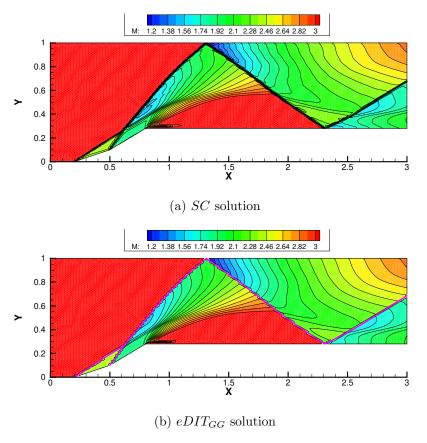
Figure 28: Supersonic channel flow: Mach iso-contours.
