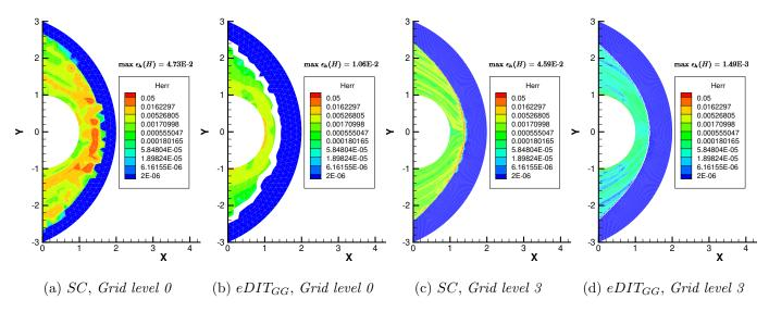
Figure 17: Hypersonic flow past a blunt body: discretization error of the total enthalpy,  $\epsilon_h(H)$ , obtained with SC and  $eDIT_{GG}$  over the entire computational domain for  $Grid\ level\ 0$  and  $Grid\ level\ 3$ .
