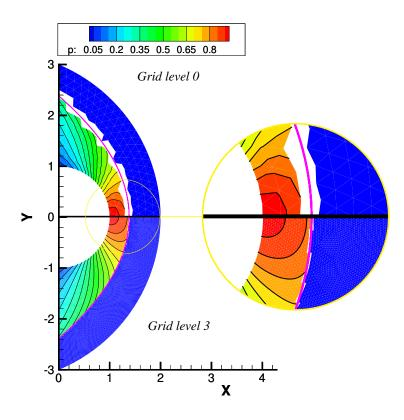
Figure 15: Hypersonic flow past a blunt body: comparison between the solutions obtained with  $eDIT_{GG}$  on  $Grid\ level\ \theta$  and  $Grid\ level\ \theta$  in terms of pressure iso-lines.
