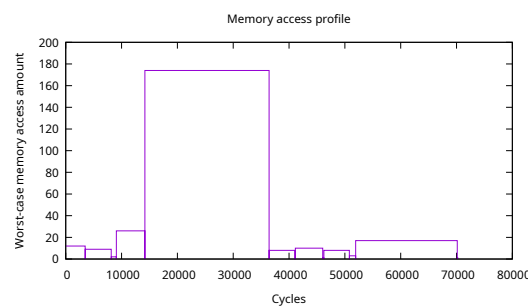
■ Figure 4 Example memory access profile ( minver , node-centric SESE regions, non-limiting large value of fuel parameter).
