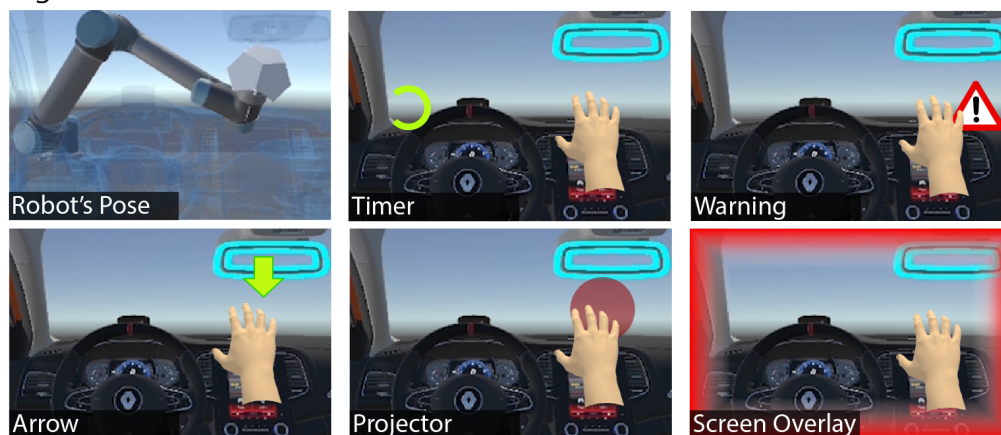
Figure 5. The signals group. This group comprises techniques that use basic signaling metaphors for displaying information about the position of the ETHD's end-effector.
