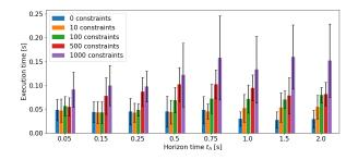
Fig. 10. Execution time of the polytope  $\mathcal{P}_x$  enumeration using ICHM algorithm averaged over 1000 executions for each of the 8 horizon lengths, with different number of added environmental constraints, ranging from 0 to 1000.
