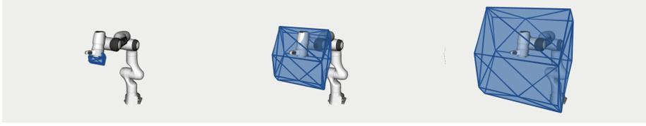
**Fig. 1.** Reachable space polytope  $\mathcal{P}_x$  for a *Franka Emika Panda* robot's end-effector for three different horizon lengths (from left to right)  $t_h = 0.05, 0.15$  and  $0.25$  seconds
