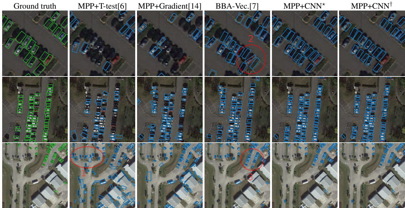
Fig. 4. Inference results for various models. For example 1: false positives, 2-3: misaligned objects
