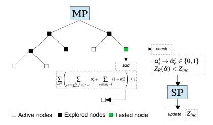
Figure 2: Single-tree Combinatorial Benders Algorithm (cut-insertion process)
