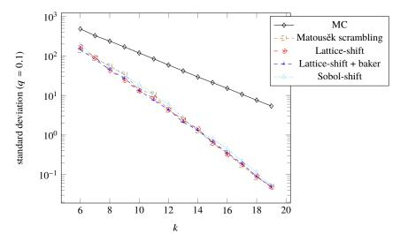
**Fig. 2** Standard deviation of array-RQMC exponential estimators as a function of  $m = 2^k$ , for the M/M/1 queue with  $\lambda = 1.0$  and  $\mu' = 4.0$  when estimating q-quantiles of hitting times to N = 10 with r = 128. For MC, we consider  $n = m \times r$ .
