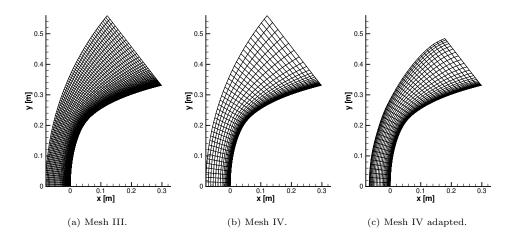
Figure 3: Numerical grids used in the study: number of nodes halved in the both the directions and effect of mesh adaptation tool.
