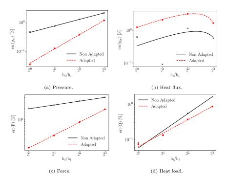
Figure 6: Relative error on the quantities of interest as function of the degree of refinement. Pressure, force and heat load in the monotonic convergence range. The observed order of convergence increases by employing grid adaption tools for pressure and force. Heat flux outside the monotonic convergence range, adaptation improves the fit.
