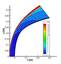
Figure 1: Mach contour at nominal condition. A strong bow shock develops in front of the vehicle to adequate the streamlines to the body shape.
