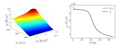
(a) Surrogate model when mesh is not(b) Angular distribution: comparison of adapted: not physical increase in the heat fluxbehaviour of adapted and non adapted is predicted for high values of free stream ve-mesh for a free stream velocity of 5600 locity and density.
