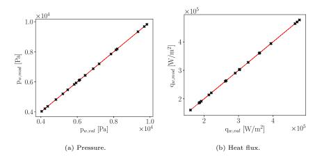
Figure 10: QQplot obtained for the adapted mesh II: the surrogate model is capable to predict correct values for the verification points.
