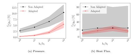
Figure 12: Ratio between the averaged grid numerical uncertainty,  $U_g(\phi)$ , and the standard deviation of the associated surrogate model,  $\sigma(\phi,h_i/h_1)$ , (solid lines), as function of the degree of refinement. Normalized standard deviation of grid numerical uncertainty,  $(S_g(\phi)/\sigma(\phi,h_i/h_1))$ , with opaque area. The numerical uncertainty is systematically lower when the mesh is adapted.
