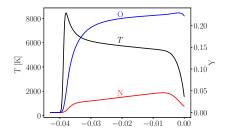
Figure 2: Temperature (left) and mass fractions (right) values along the stagnation line at nominal condition. The jump in temperature consequent to the shock drives the molecules dissociation. The resulting atoms diffuse through the boundary layer and partially recombine because of the temperature drop and the catalytic activity of the surface.
