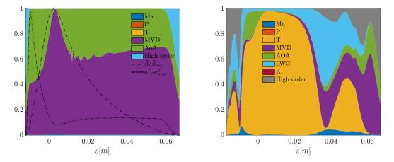
Fig. 11 Test case C. First order Sobol indexes. (a) Collection efficiency  $\beta$ . (b) Ice layer thickness B.
