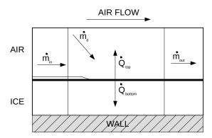
Fig. 4 Elemental domain for the computation of the ice layer thickness over the surface of interest.
