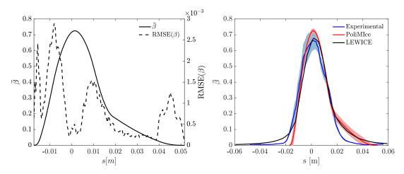
Fig. 5 Test case A. Collection efficiency  $(\beta)$  surrogate assessment. (a) Mean  $\beta$  (left scale) and RMSE (right scale) of PC predictions evaluated on the test set. (b) Comparison among numerical predictions and experimental observations. Curves are complemented by the  $2\sigma$  uncertainty obtained from PC of the computational model and experiment repeatability studies.
