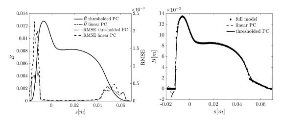
Fig. 9 Test case C. (a) Mean ice thickness and RMSE for the linear and thresholded PCE surrogates. (b) Single random PC realization. Comparison of a single PC realization, obtained for the same input, from the linear and the thresholded PC surrogates.
