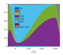
Fig. 8 Test case B. (a) Ice thickness variance w.r.t. the curvilinear abscissa. The shaded area represents the region of the airfoil surface in to which the ice accretion limits are found with input parameters varying within the preset uncertainty bounds. (b) First order Sobol indexes.
