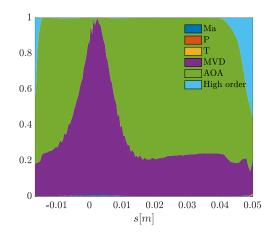
Fig. 6 Test case A. Collection efficiency  $(\beta)$  uncertainty analysis. (a) Collection efficiency variance for different PC truncation orders. The shaded area represents the region of the airfoil surface in to which the impingement limits are found with input parameters varying within the preset uncertainty bounds. (b) First order Sobol indexes.
