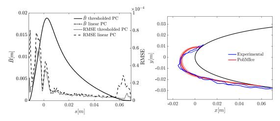
Fig. 7 Test case B. (a) Mean ice thickness and RMSE for the linear and thresholded PCE surrogates for the rime case. (b) Comparison between experimental data and computed ice shape for the NACA0012 rime case.
