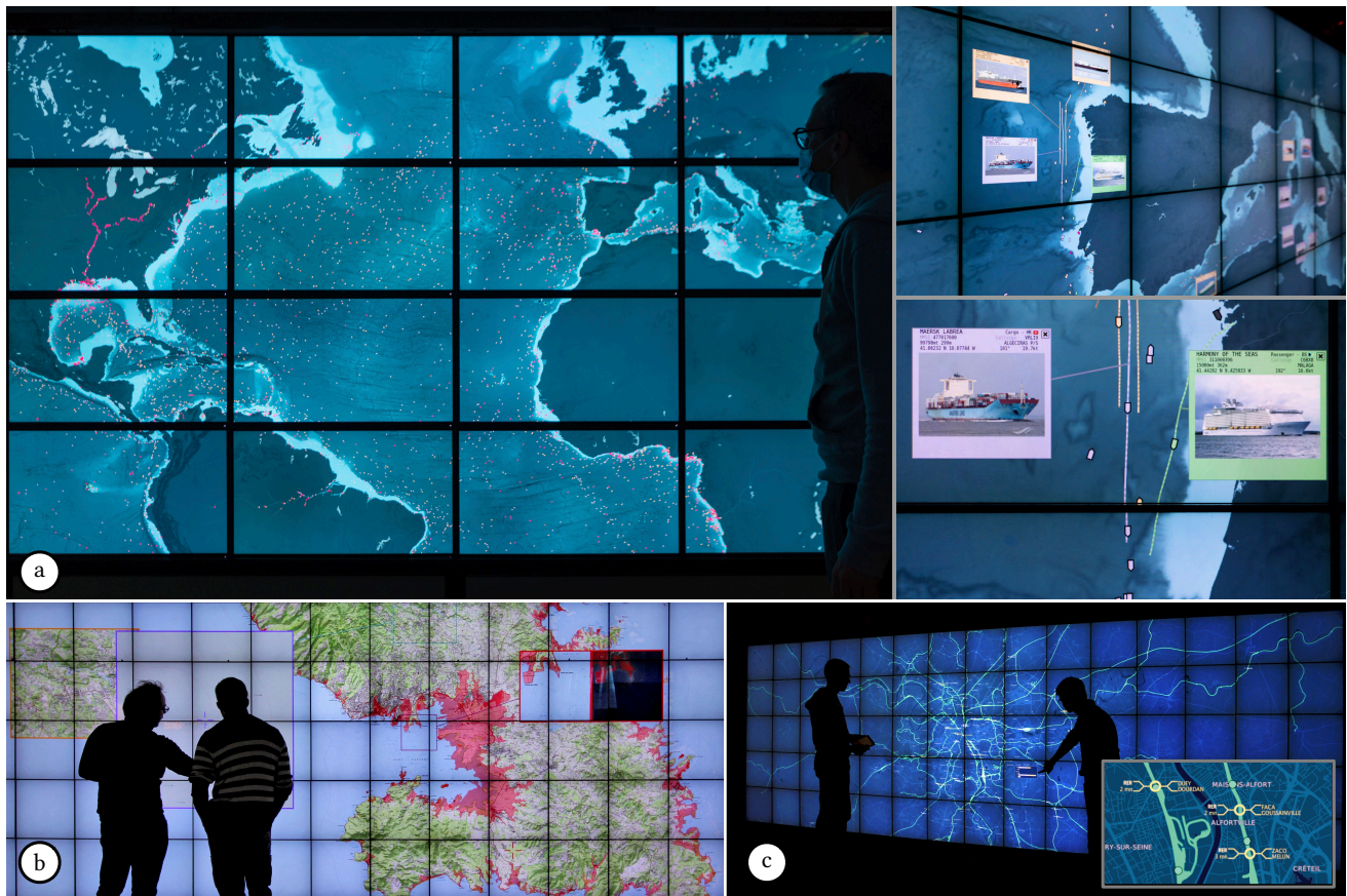
Figure 1: (a) Visualization of an AIS marine traffic data feed on the WILD-512K ultra-wall. (b) Visualization of multiple data feeds at different scales, including topographic map, ortho-imagery, sea-level rise simulation, population density data, in a crisis management scenario on the WILDER ultra-wall. (c) Visualization of a live railroad traffic feed on the same platform.
