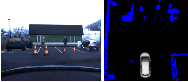
Fig. 5. On the left is an example of the visualization of an AR scene, generated from the front camera of the vehicle. On the right is the corresponding occupancy grid, seen from above. The free space is displayed in black and the occupied space in blue.
