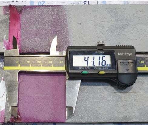
Figure 9: crack length measurement at the border of the sample.
