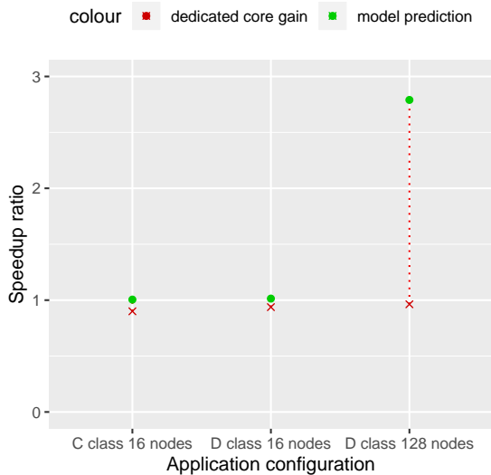
Fig. 3: Comparison of the model prediction and the dedicated core case (Speedup to the time with no progression) for NAS BT-MZ for different configurations on inti/sandy-bridge .
