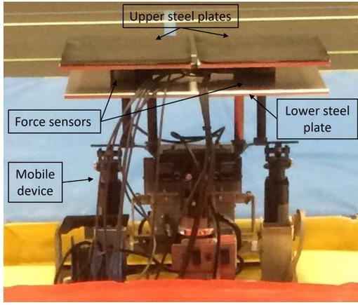
Fig. 1. Force platforms fixed on the mobile device
