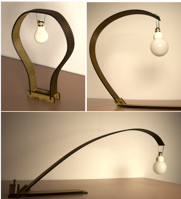
Figure 11: Laser-cut bending-active structures made of MDF panels.
