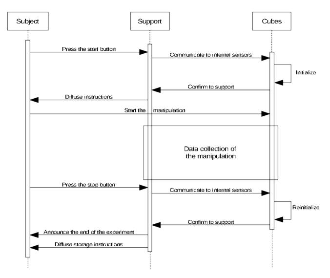
Figure 3 : UMLSequence diagram of the activity representing the timeline of interactions.
