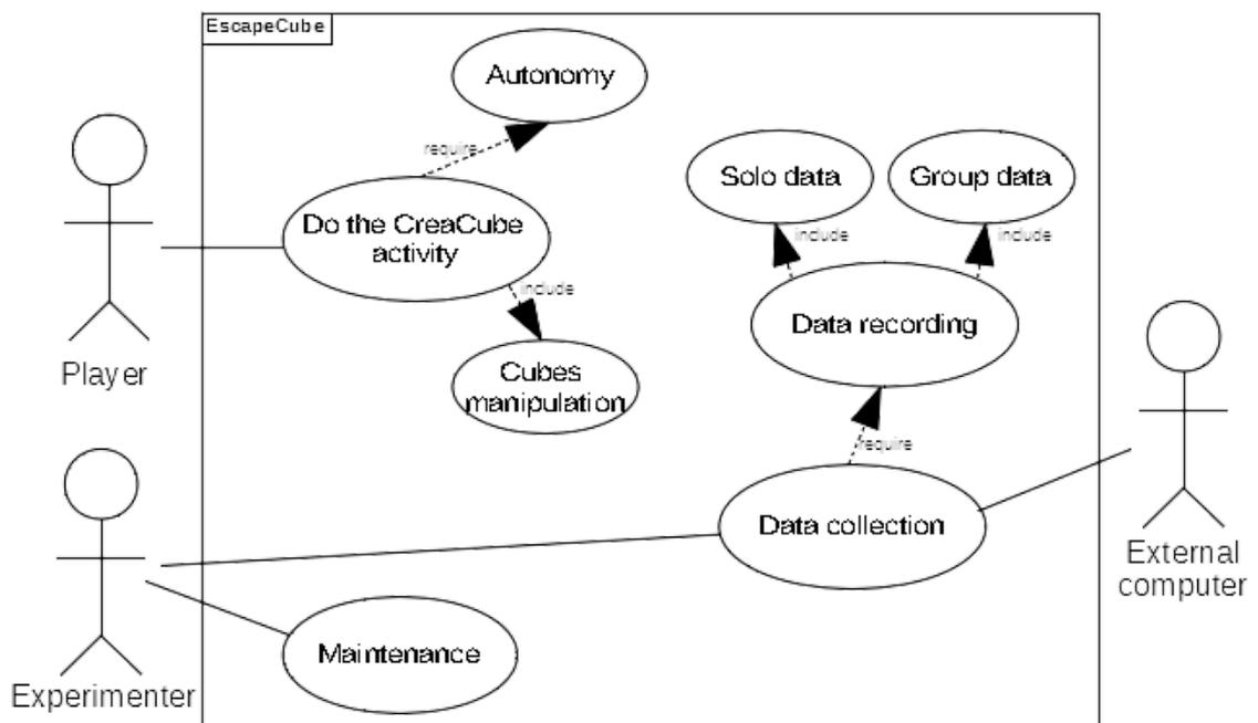
Figure 2 : UML Use-case diagram of EscapeCube
