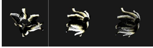
Fig.14. Flower point cloud after registration by ICP algorithm
