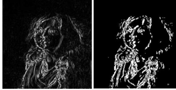
Fig. 5. The left picture shows the effect picture of edge detection, and the right picture shows the effect picture after morphological operation
