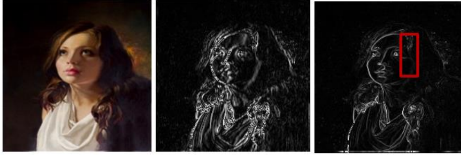
Fig. 3. Original image and Effect diagram of Sober operator and Prewitt operator
