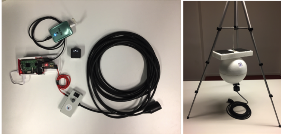
(a) Microcomputer with the power bank, Wi-Fi dongle (b) Assembled buoyant cap for communication with GoPro, audio jack and stereo cable, and a hydrophone. Tripod is used for exhibition.
