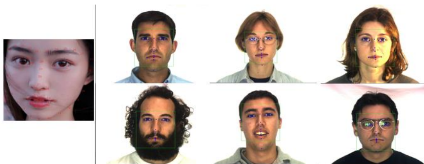
Fig 2. The single face on the left represents the pre-defined dlib shape landmarks. On the right the pipeline's result is shown i.e. a bounding box and the relevant landmarks.
