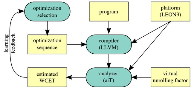
Figure 1: Iterative WCET-oriented compilation workflow (from [7])
