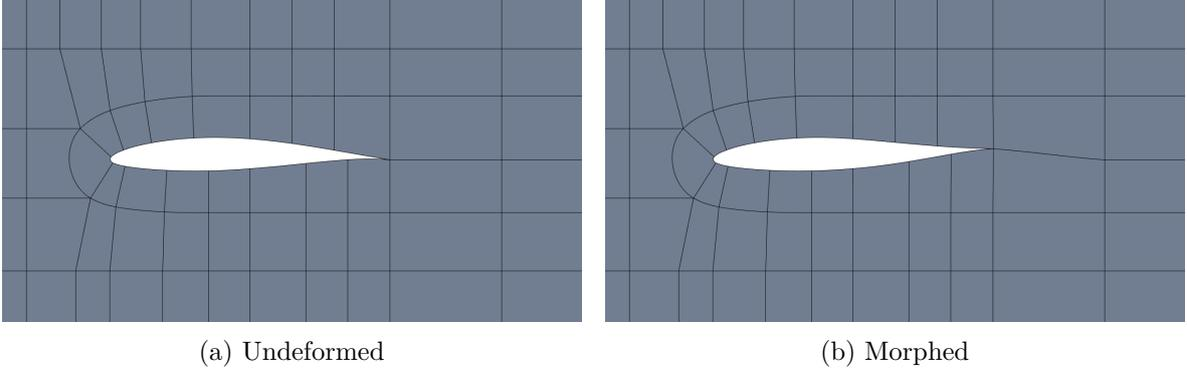
Figure 18: Primary mesh around the morphing airfoil
