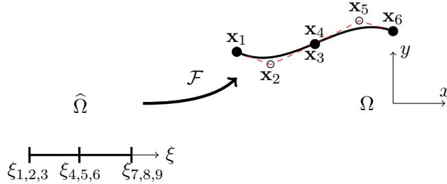
Figure 4: Example curve of figure 2 after Bézier extraction procedure.
