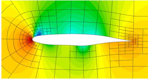
Figure 16: Optimal shape (adapted mesh and density field).
