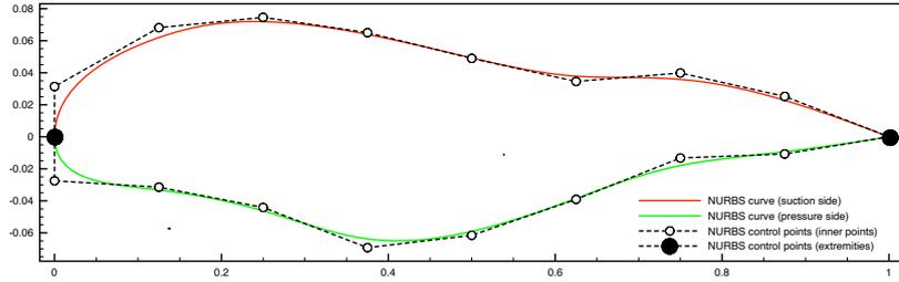
Figure 6: Airfoil geometry defined by two NURBS curves.
