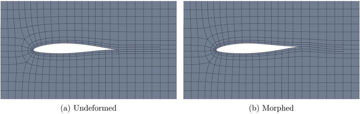
Figure 19: Secondary mesh around the morphing airfoil
