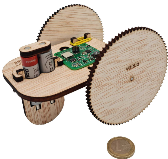
FIGURE 1. DotBot: a low-cost, micro-robot for educational and research purposes in networking and swarm robotics.
