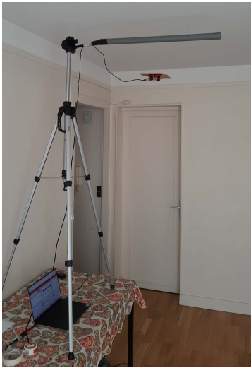
FIGURE 7. BOOSTXL-AOA angle of arrival estimation test setup.
