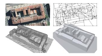
**Figure 8:** Result on a building block. The output 3D model (bottom right) obtained from a multi-view stereo point cloud (bottom left) preserves the main roof components while ignoring small elements such as chimneys and dormer-windows.
