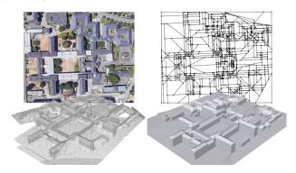
**Figure 9:** Result on a large regular building. Our 3D output model (bottom right) preserves the orthogonality existing between facade and rooftop components. Note how the planimetric partition (top right) aligns well with the aerial image (top left, not used).
