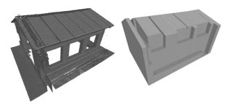
**Figure 11:** When running the pipeline on a building that does not verify the 2.5D hypothesis, the piecewise-linear modelling cannot represent the building correctly and leads to overly complex representations, as different heights of the building project on the same 2D cells (roof and opening for example).
