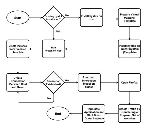
Figure 6. Traffic generation using Firefox.
