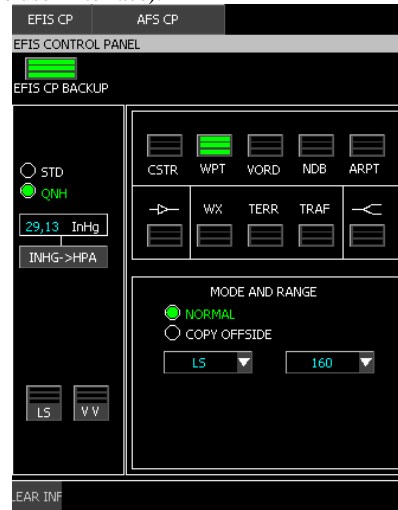
Figure 18 : EFIS control panel (left panel is highly critical DAL A while right panel is less critical DAL C [63])
