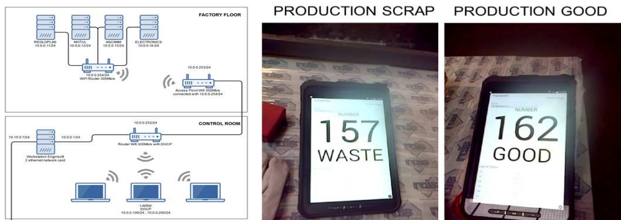
Fig. 4 – LAN network connection and real time prediction of Waste and Good castings shown on tablet
