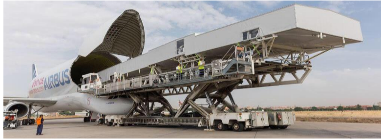
Fig. 2. The transportation jig during loading at the Airbus Beluga.
