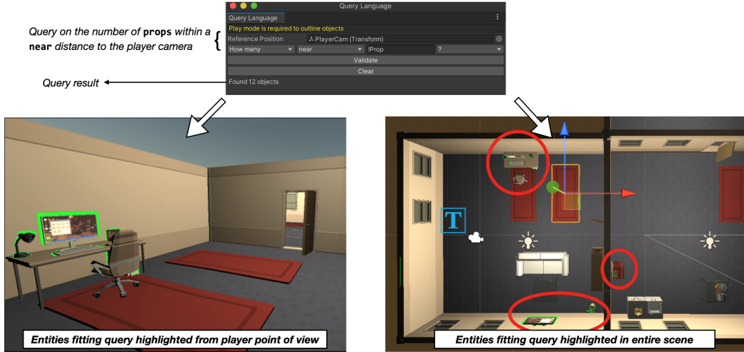
Fig. 10. Here we show the window to construct a simple query using the syntax from Figure 6 that counts the number of props within a near distance (3 meters) of the player camera. The two views show the highlighting in the scene from the player viewpoint (left) and the Unity scene view from above (right).
