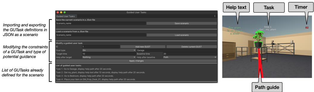
Fig. 8. (Left) This interface allows designers to define GUTasks , add and edit task constraints, view the list of existing tasks. The tasks can be easily loaded and exported in the GUST-3D representation for reuse in various scenarios. (Right) The tasks are communicated to the user in real time, and additional help text and path guidance can be provided at a fixed time point. The timer indicates seconds past.
