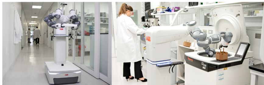
Fig. 4. Assistive, collaborative AMR in a hospital laboratory [14]
