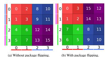
Figure 4: HFP's processing order on a Square 2D Matrix Multiplication with M = 4. The colored lines on the sides represent data loads of rows or columns for the tasks of the corresponding color.
