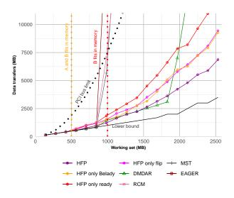
Figure 7: Amount of data transfers on the Square 2D Matrix Multiplication in real execution with 1 Tesla V100 GPU, N ranging from 5 to 90.
