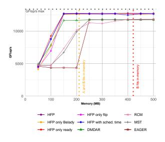
Figure 6: Performance on the Square 2D Matrix Multiplication in real execution with 1 Tesla V100 GPU while varying the memory size, N set to 15
