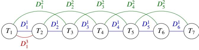
Figure 2: Data sharing among tasks that reach worst-case complexity for HFP (depicted for  $m = 7$ : an edge between two tasks represents a data shared by these tasks. Note that in addition to these data, tasks have private data so that each task exactly has  $\Delta$  input data (except for  $T_m$  with  $\Delta - 1$  data).
