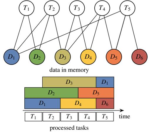
Figure 1: Example with 5 tasks and 6 data, with a memory holding at most  $M = 3$  data. The graph of input data dependencies is shown on top. The schedule below corresponds to processing the tasks in the natural order with the following eviction policy:  $\mathcal{V}(1) = \mathcal{V}(2) = \emptyset$ ,  $\mathcal{V}(3) = \{1\}$ ,  $\mathcal{V}(4) = \{2\}$ ,  $\mathcal{V}(5) = \{3, 4\}$ . This results in 7 loads (only  $D_1$  is loaded twice).
