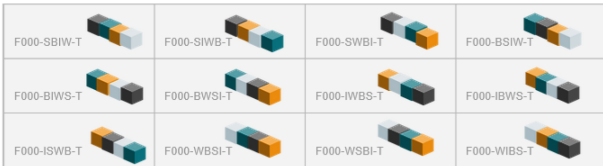
Figure 4 : 12 configurations for the F000 structure detailed by (Mercier et al., 2022). The configuration is coded by four letters S (sensors), W (wheels), B (Battery) and I (inverter), and the letter T (or F) indicates if the structure can be a goal-structure, depending on the orientation of the wheels and the sensor, and if the switch is turned on.
