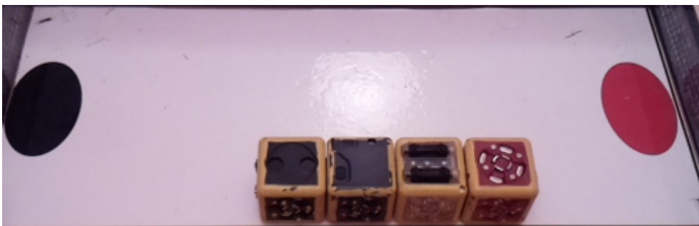
Figure 1 : An example of configuration of CreaCube. The four cubes must be assembled in order to make them move autonomously from the red point to the black point
