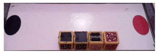
Figure 1 : An example of configuration of CreaCube. The four cubes must be assembled in order to make them move autonomously from the red point to the black point
