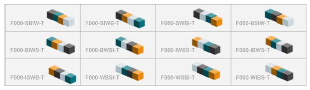
Figure 4: 12 configurations for the F000 structure detailed by (Mercier et al., 2022). The configuration is coded by four letters S (sensors), W (wheels), B (Battery) and I (inverter), and the letter T (or F) indicates if the structure can be a goal-structure, depending on the orientation of the wheels and the sensor, and if the switch is turned on.
