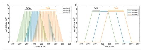
Fig. 2. Signals sent to the three actuators in the two actuation modes. A) Vibratory mode, made of sinusoïdal oscillations at 120 Hz within ramp envelopes. B) "Tap" mode made of single ramp signals. In this Figure, we used DoS = 220 ms and SOA = 110 ms.
