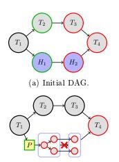
(b) Execution of  $H_1$  (i.e. submission of the corresponding task graph).  $H_2$  is not processed yet.
