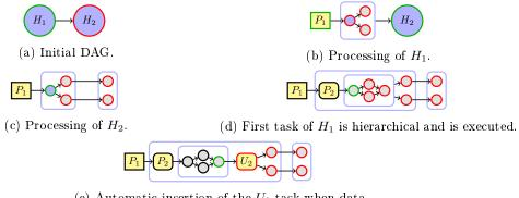
(e) Automatic insertion of the  $U_2$  task when data needs to be accessed.
