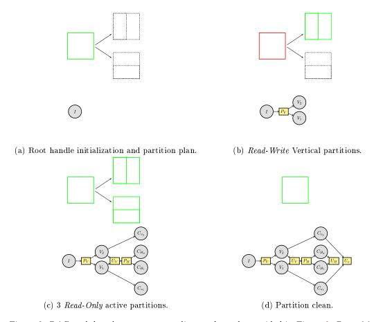
Figure 3: DAG and data layout corresponding to the code provided in Figure 2. Dotted border stands for *inactive*, solid border stands for *active*. Red border stands for *read-write partitioned*. Green border stands for *read-only partitioned* or *unpartitioned*.
