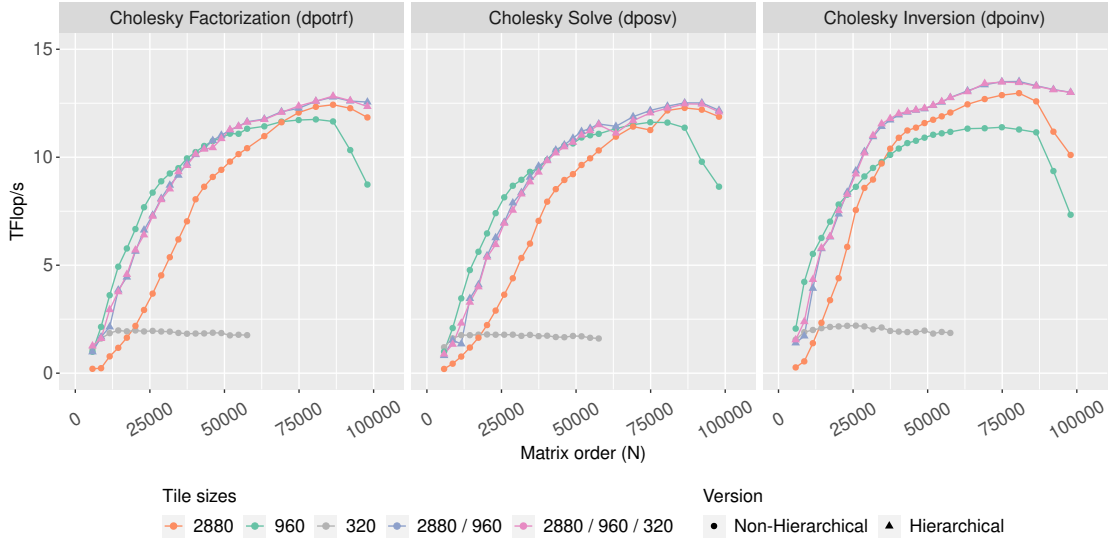
Figure 10: Comparison of the hierarchical strategy to the original one on Cholesky type operations (DPOTRF, DPOSV, DPOINV) kernel with diagonal distribution of the hierarchical tasks.
