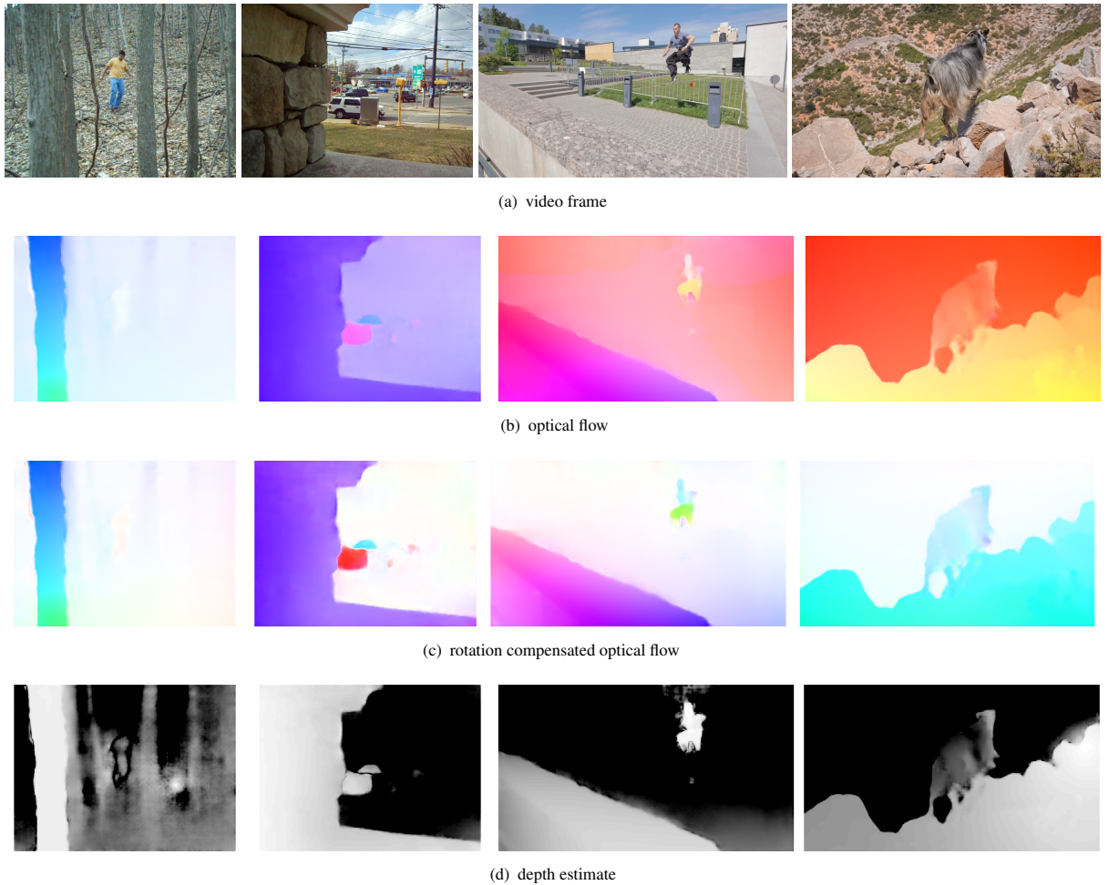
Fig. 7 Flow, rotation compensated flow and the relative depth estimate. We show sample videos from the data set Complex Background (video sequences: traffic, forest) as well as two sample videos from the Davis data set (video sequence: parkour, goat). A comparison of (b) and (d) shows how motion at distant is dominated by camera rotation. After subtracting of the camera’s rotation the remaining flow magnitude in these areas is very small (light color). If the flow magnitude is small the motion direction is noisy. This can be seen in (e).
