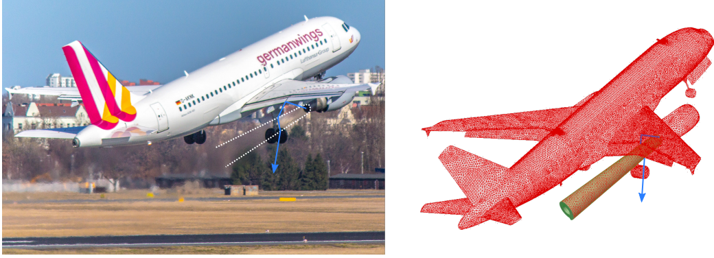
FIGURE 2: An acoustic wave (blue arrow) emitted by the aircraft’s engine, reflected on the wing and crossing the jet flow. Real-life case (left) [23] and a numerical model example (right). The red surface mesh represents the aircraft’s surface and the surface of the green volume mesh of the jet flow.
